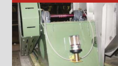
Fan lubrication in food industry
